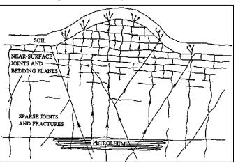
Possible microseepage paths up through the network of fractures, joints and bedding planes
